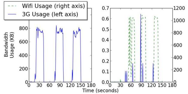
Figure 4: Bandwidth (3G-only vs. 3G + Offloading)
