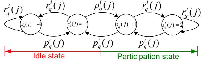
Fig. 5. An example of the Gur Game with associated memory size  $M = 2$ , where positive number states give the corresponding output of the contextual information for user  $i$ , e.g., text message, low resolution image, or high resolution image. Negative numbers state represent ‘no participation’ decision of the user.
